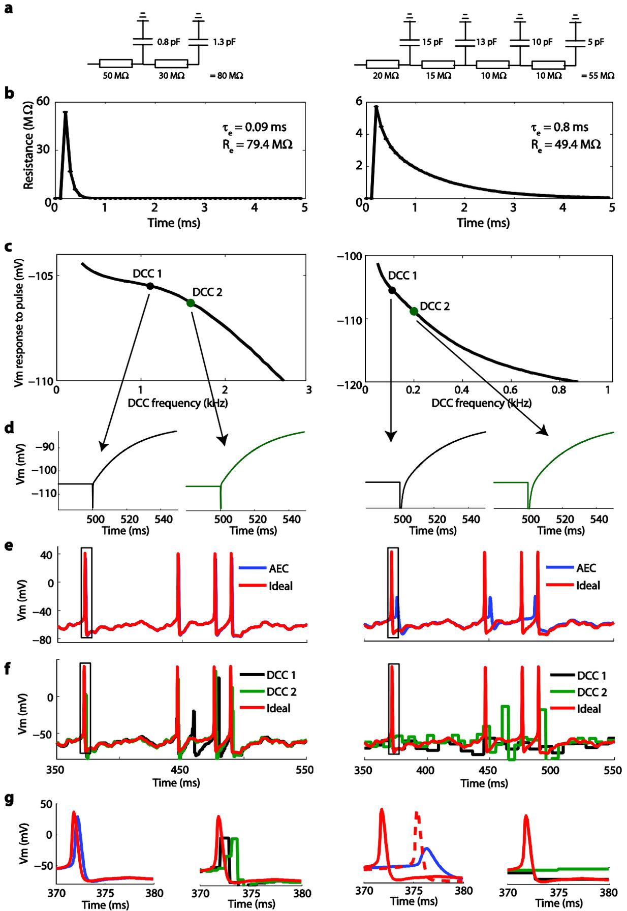
Left column : with a fast electrode made of two resistors and capacitors (time constant 0.09 ms from exponential fit); right column: with a slow electrode made of four resistors and
